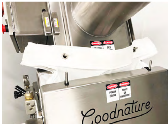
Fig 3.1: Press bag in grinding position
