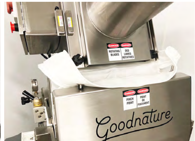
Fig 3.2: Press bag in pressing position
