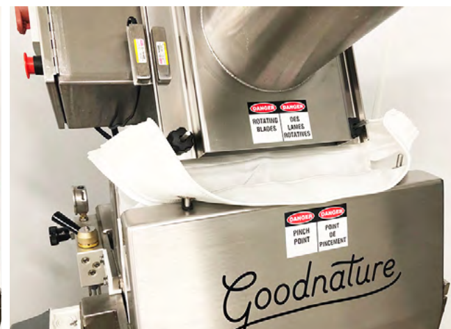
Fig 3.2: Press bag in pressing position
