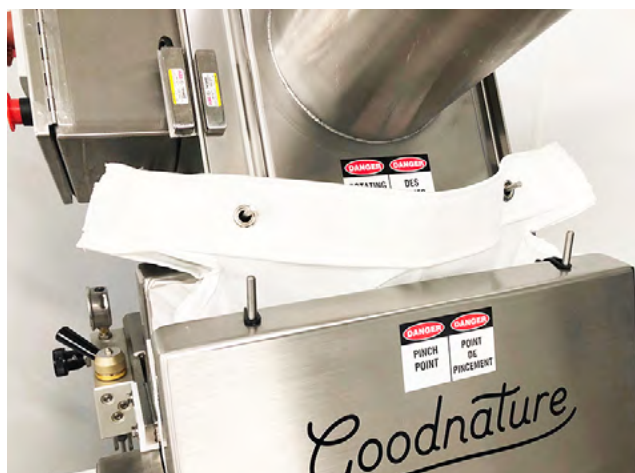
Fig 3.1: Press bag in grinding position
