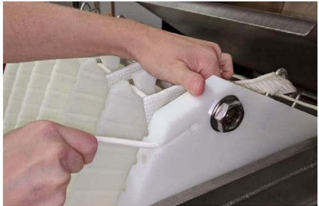
*Fig 4.6: Rubber Cord into Rack Slot*
