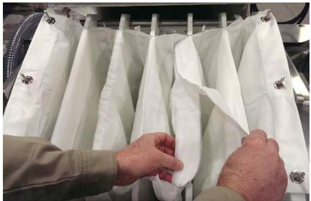
*Fig 4.4: Attaching bags by Velcro*
