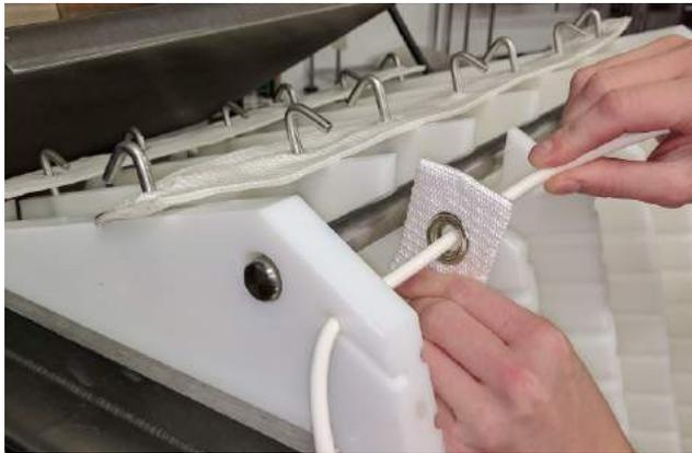
*Fig 4.5: Threading the Rubber Cord*
