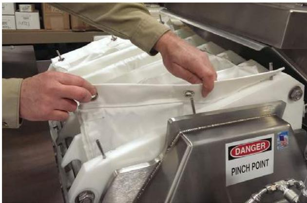
*Fig 4.3: Installing press bags over pins*
