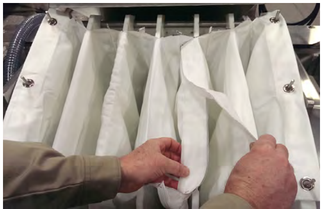
Fig 4.4: Attaching bags by Velcro
