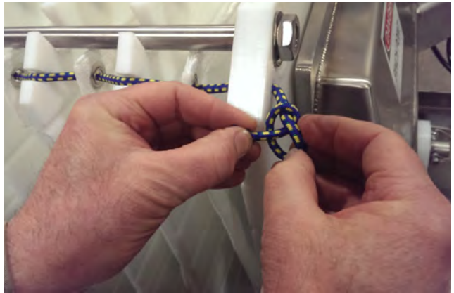
Fig 4.6: Knotting the Bungee Cord
