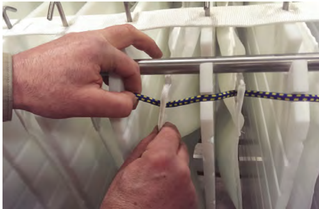
Fig 4.5: Threading the Bungee Cord
