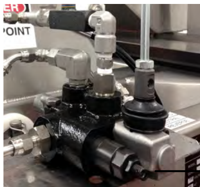
Fig 5.3: Adjusting Hydraulic Pressure
