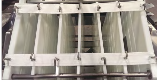
Fig 4.2: Installing press rack straps
