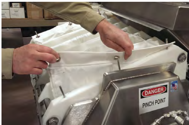
Fig 4.3: Installing press bags over pins
