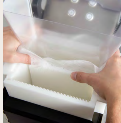
Carefully insert Bag Separator against first funnel, making room for second funnel to be inserted.
