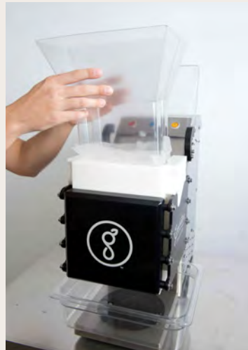
This image shows removal of the Loading Funnel after adding shredded produce.
